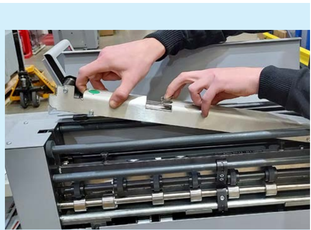
Removing the 'EasyBlade' safety cover.
